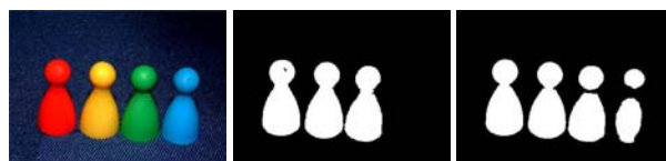
Fig. 4. Illustration of segmentation based on ROI. The original image lies on the left, the mask generated by the Achanta model is in the middle, and the proposed model produces a mask on the right.
